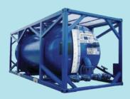
ASME pressure vessel and lined with Epoxy Flakes or LDPE lined to ensure safe transportation of corrosive cargoes. Equipment is design & build as per the IMDG code and rated at T14.
