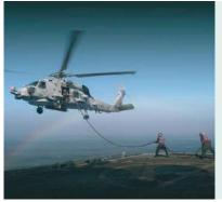
Protank HIFR Assembly is fully compliant with STANAG 3847. This is a low pressure loss assembly which is designed for ship to helicopter refueling. The assembly is manufacture in facility in Malaysia, with the option of two end configuration;
