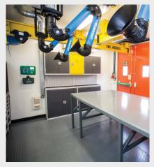
17ft DNV 2.7-1, A0 Safe Area (Pressurised) Fabrication Workshop complete with overhead fixed and retractable trolley beams, heavy duty fabrication work benches, storage cabinets for tools and equipment, fume extraction system c/w flexible fume extraction arms.
