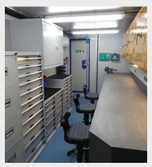
20ft DNV 2.7-1, Non rated Safe Area Workshop complete 7kW A/C System, storage cabinets for tools and equipment, work bench and workstations.
