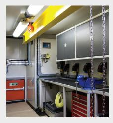
20ft DNV 2.7-1, A60 Zone 2, Wireline Workshop Container complete with 7kW A/C System, overhead retractable trolley beam, work bench, workstations, tool racking, storage cabinets for tools and spares.
