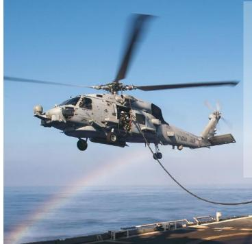
Protank HIFR Assembly is fully compliant with STANAG 3847. This is a low pressure loss assembly which is designed for ship to helicopter refuelling.
